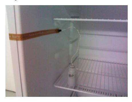
Step 4: Connect the sensor to the flex tape on the inside of the fridge.
