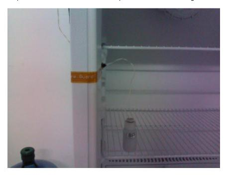
Step 5: Use the included connector cable to go from the flex tape to the Temperature Guard monitor.
