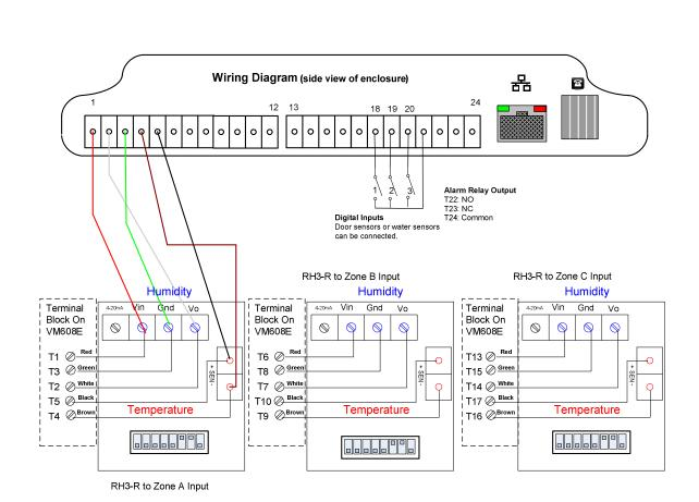
The terminal blocks on the front of the enclosure are removable. To remove a terminal block pull straight out.
