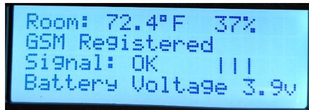
This screen displays the internal sensor current temperature and humidity, cellular module status, signal strength, and battery voltage after pressing the cancel alarm button once.
