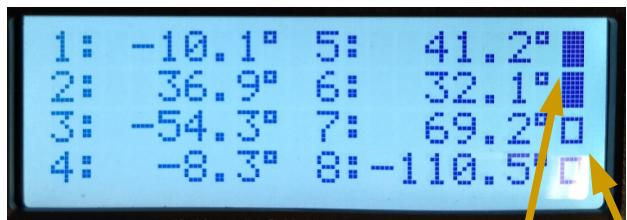
The dry contact inputs are on the right side of the display of the main screen. The closed square means the input is **closed**, an **open** square is an open input. Top square is Input #1, second is Input #2 etc. If the input is set to water sensor, the open square is no water detected, the closed square is a wet condition. The inputs are not displayed in the scroll through menu unless they are in alarm.
