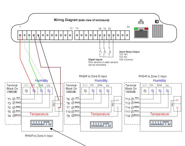
If humidity reading is way off or not recognized, check to make sure dip switches 6 and 7 are in the up position.
