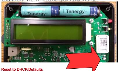
Unplug the unit while it is on. Hold down the Reset Defaults switch, while plugging it back in. As soon as the LED1 comes on release the Reset\_Defaults switch immediately. Unit will now be in DHCP mode. This actually resets the network adapter to defaults. If the LED1 keeps blinking instead of going solid on, reboot with the power switch.
